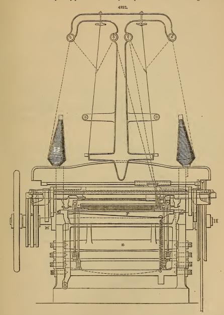
These are shown half size in Fig. 4854, and enlarged details are given twice full size in Figs. 4856 to 4863. The five primary parts are the thread-tube delivering the thread, the sinker, the needle, the knocking-over bit, and the coverer. The action will first be explained of these five primary parts which manipulate the thread, and then of the secondary parts which effect the movements of the primary parts.
